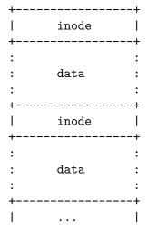
That's it, each inode describes a block of data of variable size that immediately follows. Then more pairs of inode-data follow until the end of the device. However, a requirement is that each inode has to be aligned to 128 bytes.
